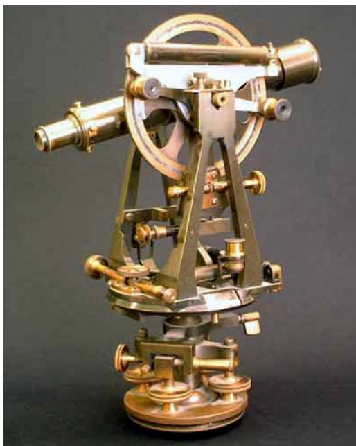
Troughton and Simms theodolite Ca 1880, similar to the type of theodolite that Turner would have used.
